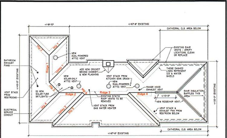
1986 SUNNYSIDE DRIVE - ROOF PLAN SCALE: 1/4" = 1'-0"
